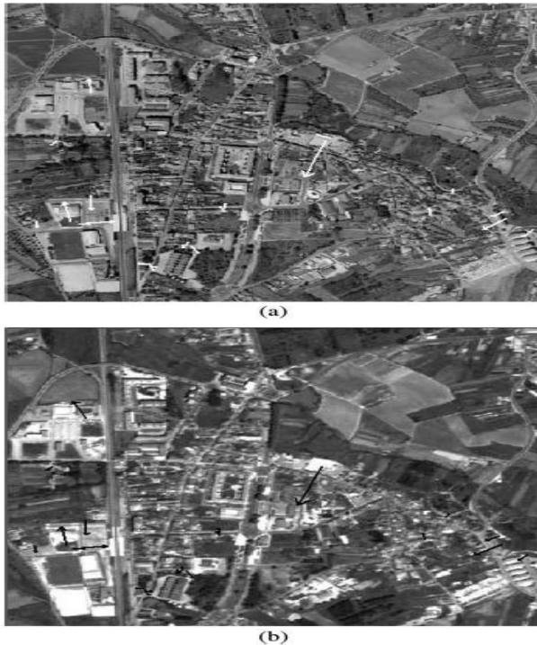
Fig. 11. (a) Segment (reference) with 512 \times 512 pixels from the first principal component of the orthophotograph. (b) Segment with 512 \times 512 pixels from an ALOS-PRISM scene. The final set of keypoints (location, scale, and orientation representation) used for registration is superimposed on both images for d_{ratio} = 0.9 . Further details are given in Section III-D.
