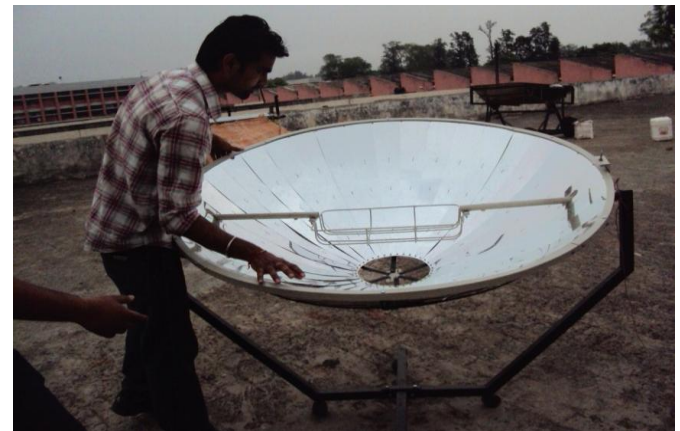
Figure 3: Experimental diagram of the parabolic dish collector.
