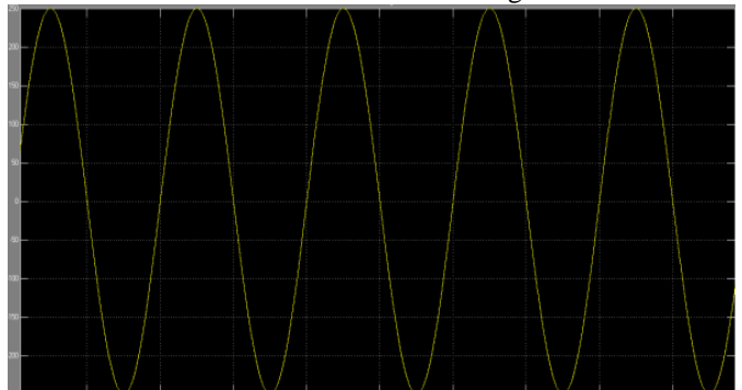
Fig.13. Input supply voltage.
