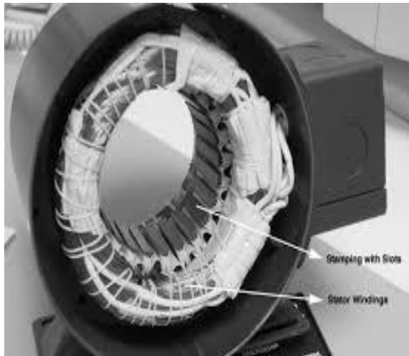
Fig.1. BLDC motor stator construction.
