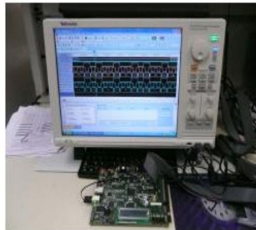
Fig. 4. Test setup showing the Logic Analyzer and Spartan 3E development board.
