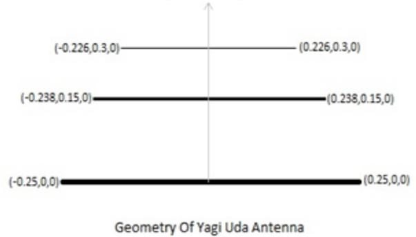
Fig.1. Geometry of Yagi Antenna.
