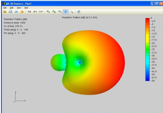
Fig.4. Radiation pattern in dB.
