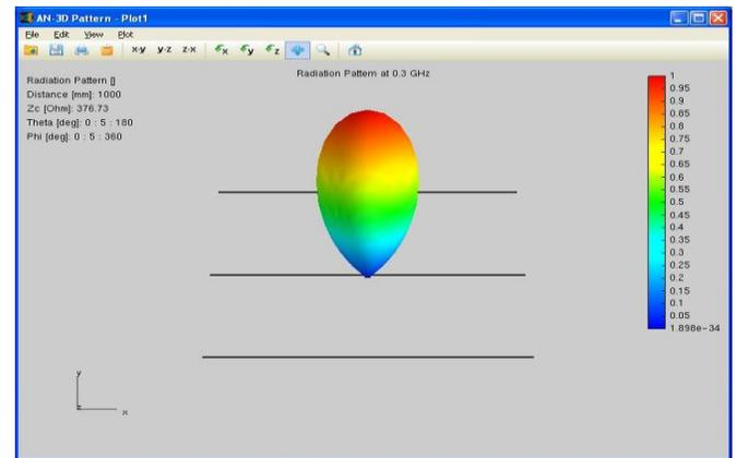
Fig.3. radiation pattern of Yagi antenna.
