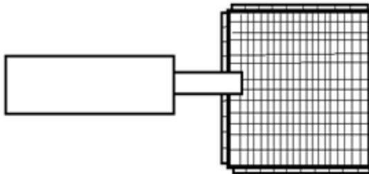
Fig.5. Geometry of dual band microstrip antenna.
