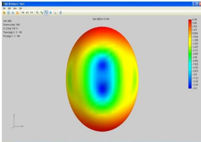
**Fig.8. Gain in dB of dual band microstrip antenna.**
