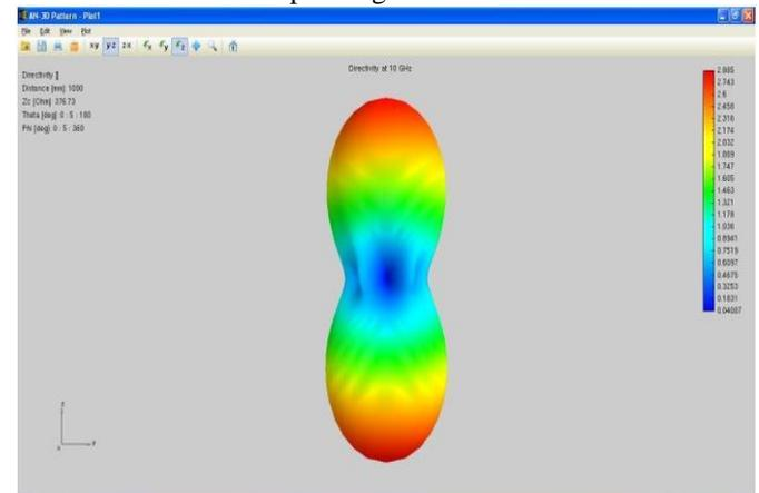
Fig.7. Directivity of dual band microstrip antenna.
