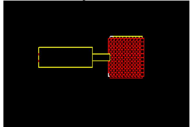
Fig.6. Simulated dual band microstrip antenna.
