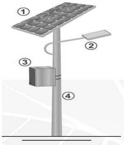
Fig.5. Schematic representations for the structural composition of a PV LED lighting system.
