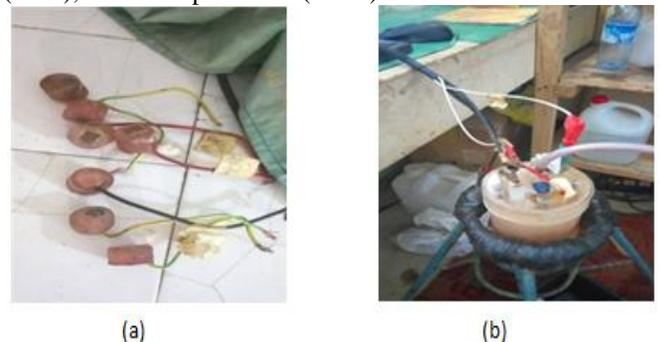
**Fig 3: (a) Working electrodes and (b) Experimental set up for electrochemical process.**
