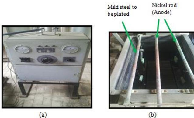
**Fig2: (a) Greasing chamber and (b) Setup of the plating bath process.**
