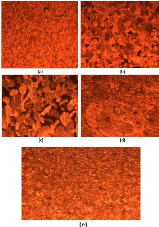
Fig 4: Micrograph showing (a) as-received (b) tempered (c) annealed (d) normalized (e) hardened mild steel microstructures (× 200 magnifications).
