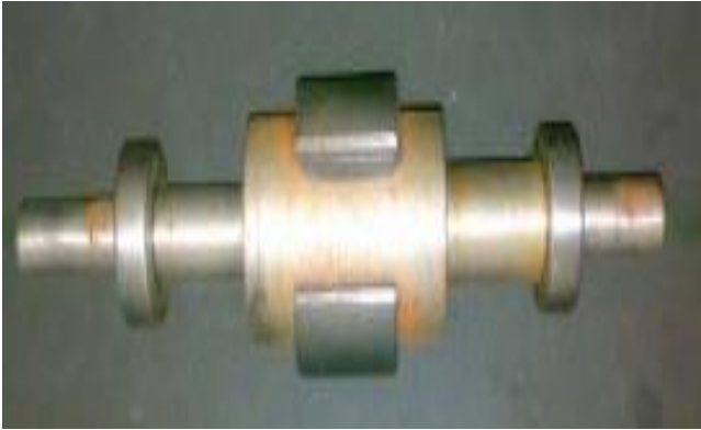
Fig.3. Mounted magnet on the rotor shaft.
