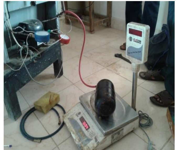
Fig.10. Charging of LPG.
