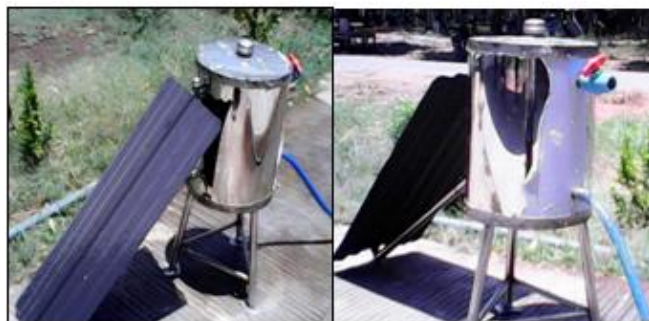
Fig.2. photo of constructed thermal storage system.
