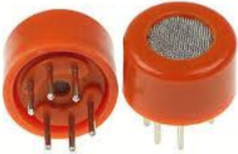
**Fig.6. Alcohol sensor.**
