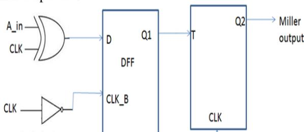
Fig8. Block Diagram of Miller Encoding.
