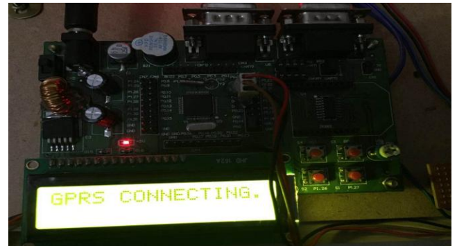
Fig.8. GPRS tracking system is connecting to post output values in website at unique address.
