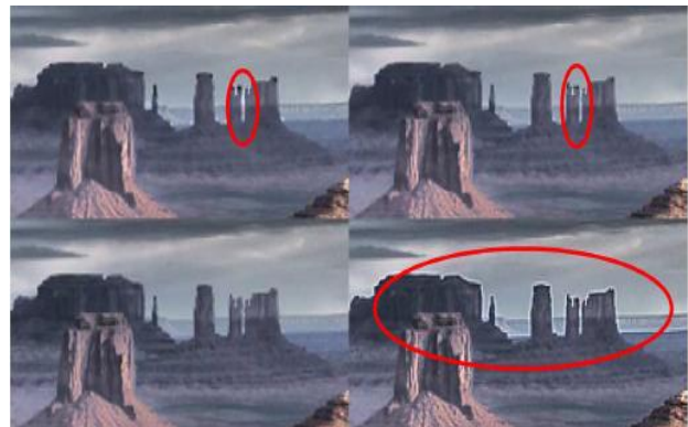
Figure5. Results of the proposed algorithm using (3x3) mask with different shapes. Top left: square shape. Top right: diagonal cross. Bottom left: horizontal/vertical cross. To illustrate the halo-effect, a linear filter with a (3x3) uniform mask is used to replace the median filter in the proposed algorithm. The result is shown in the bottom right. The halo-effects are marked by red ellipse.
