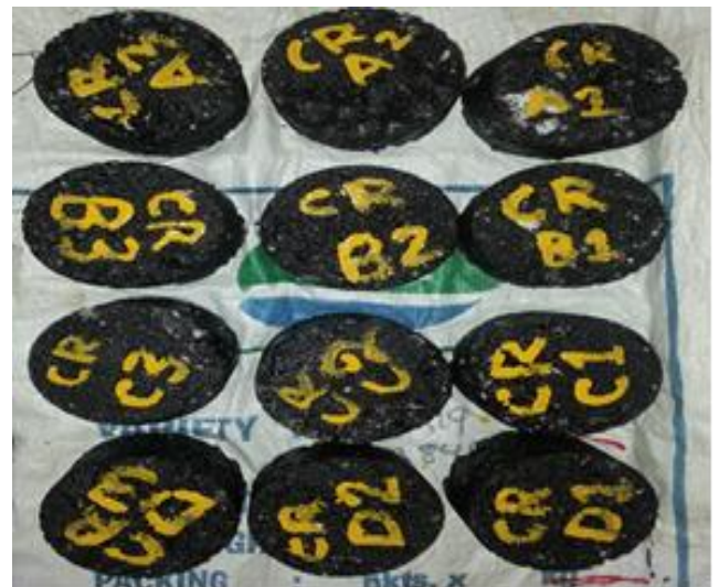
Fig.5: Marshall moulds using Crumb Rubber Modified Bitumen.
