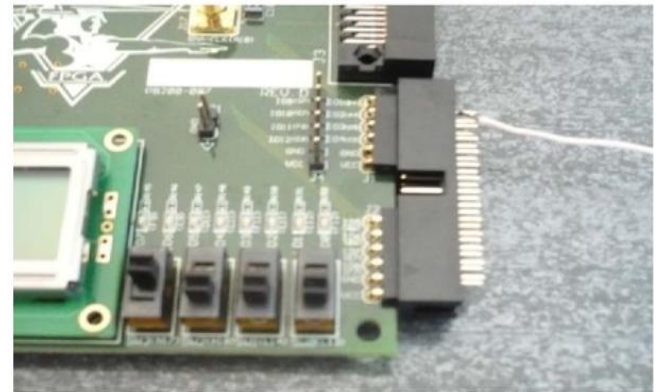
Figure14. The slide switches and the connector which makes the junction between the pulse generator and the board.
