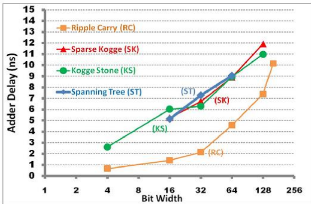
Fig.12. Measured results for the parallel-prefix adder designs compared with the RCA.
