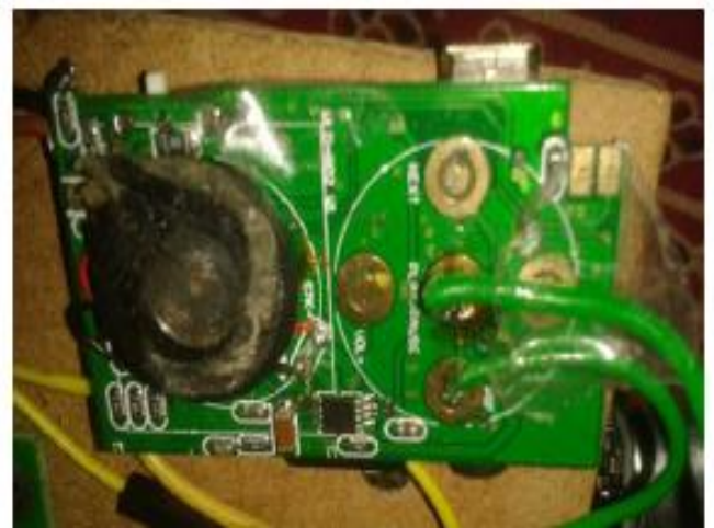
Fig.10. MP3 player interfaced with microcontroller
