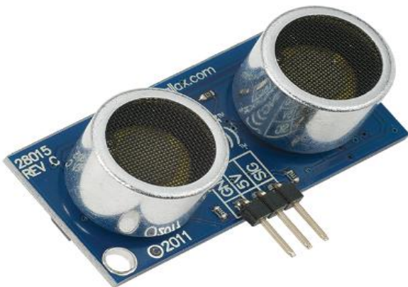
Fig.5. Basic structure of Ultrasonic sensor.
