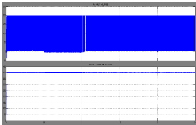
Fig.10 PV Input & Output Voltages.
