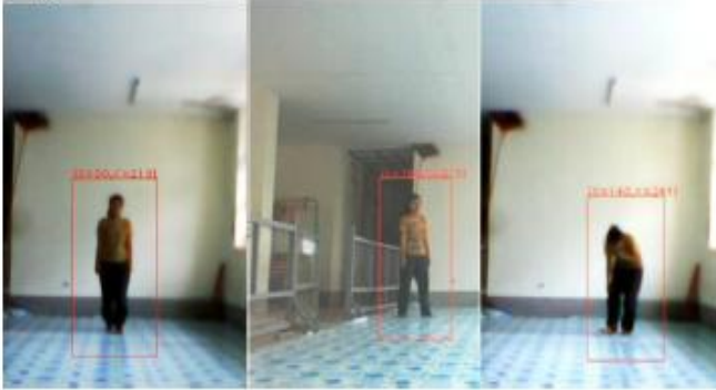
Figure5. Pedestrian Detection using HOG and SVM.
