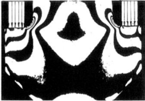
Fig.5. Stress concentration in fillet of T-root.
