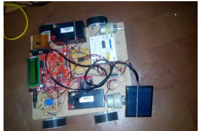
Fig.6. best battery charging using solar energy for robotic vehicle based on relay host microcontroller without power supply.
