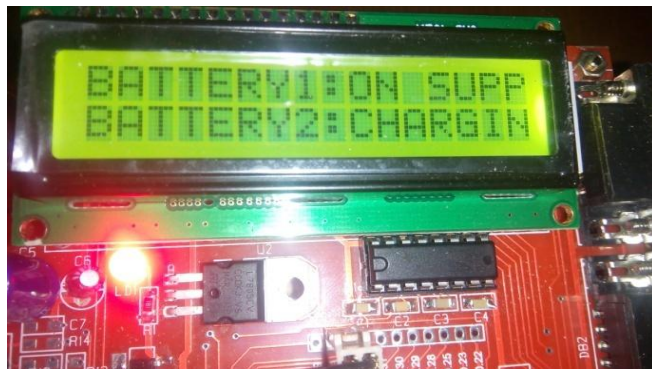
Fig.9. Charging the Second battery with the solar power displayed on the LCD.
