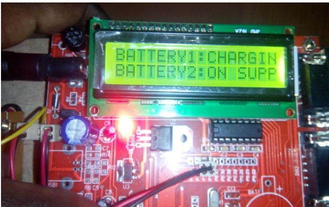
Fig.8. Charging the first battery with the solar power displayed on the LCD.
