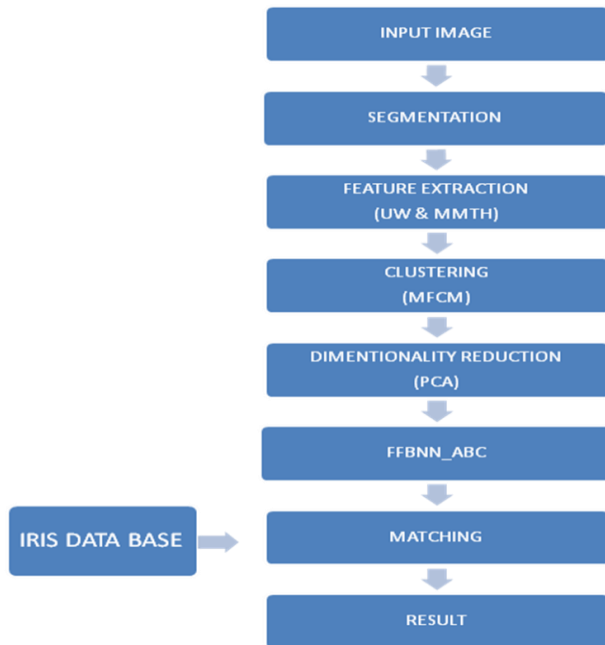
Figure1: Architecture of Our proposed Iris Recognition System.
